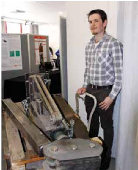
Rather than cutting through the vehicle, Andrew's Car Spreader is designed to straighten bent steel back to its original shape.
