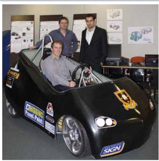
A single-seater battery-powered electric vehicle was just one of the outstanding engineering design projects on show at the University of Waikato in October last year.
