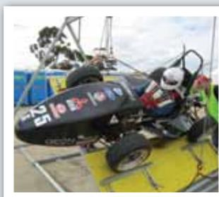
Waikato's 2010 Formula SAE race car is tested for leaks and stability at the 2010 competition.
